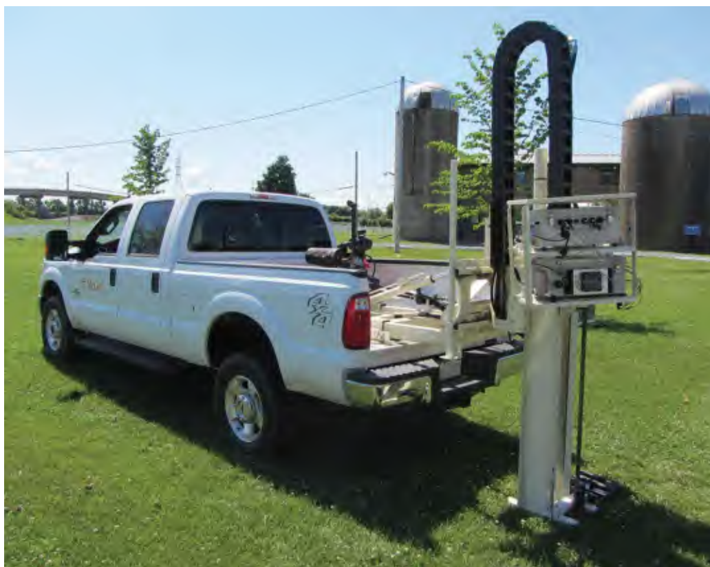
A probe equipped with insertion load sensors and two spectrometers, which cover visible and near infrared parts of the spectrum as well as electrical conductivity.
